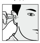
2. Grip the plastic handle of the Rocket plug and slide the plug into the ear canal. Rotating the plug slightly whilst inserting may help.
